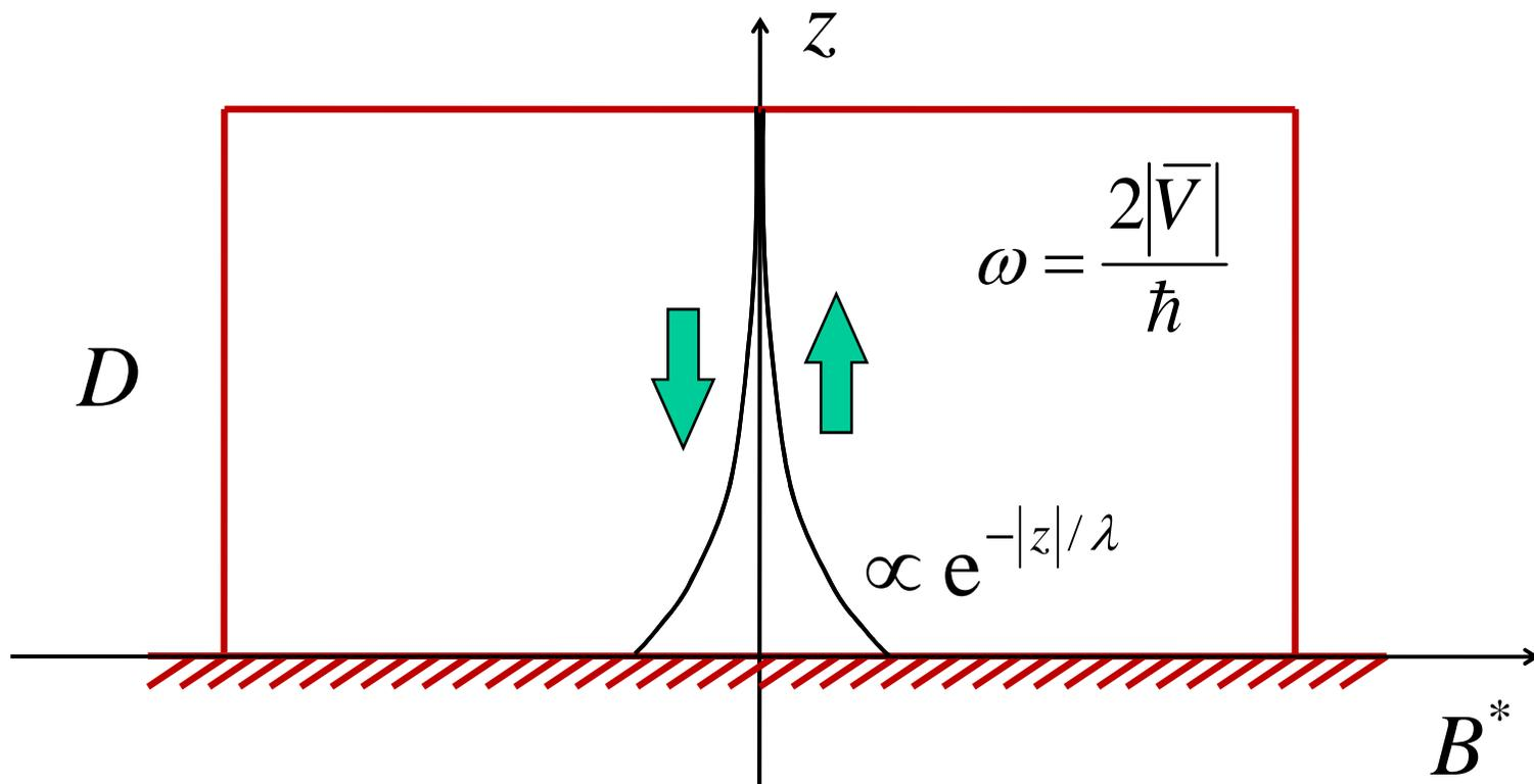
$$\bar{V} = \pm \frac{1}{D} \int_0^D V(z) dz = \pm \frac{\hbar^2}{4m} N \frac{1 - e^{-D/\lambda}}{D} g_s g_p \lambda^2$$
