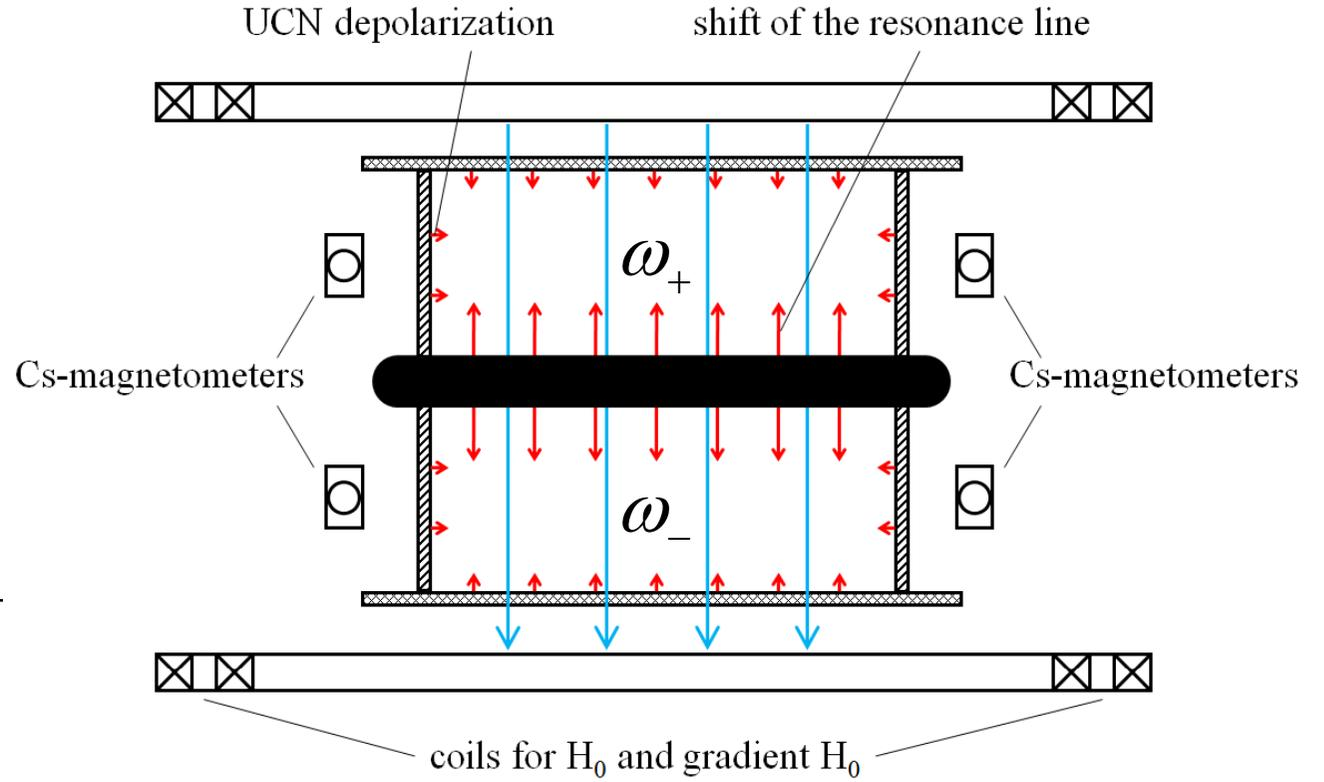
$$\Delta_{\pm} \omega = \omega_{+} - \omega_{-} = \frac{4|\bar{V}|}{\hbar}$$
