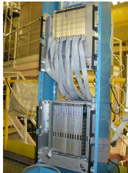
UCN detector with analysis of polarization (13 neutron channels, 117 Si detectors with electronics)
