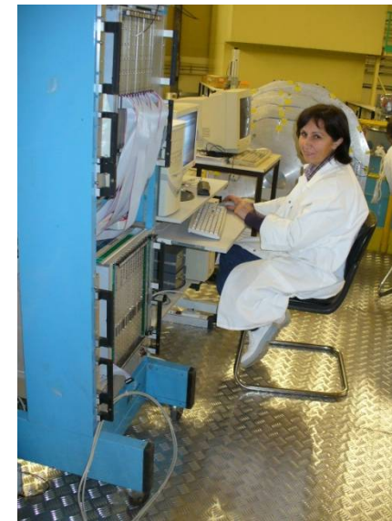
UCN detector with analysis of polarization (13 neutron channels, 117 Si detectors with electronics)
