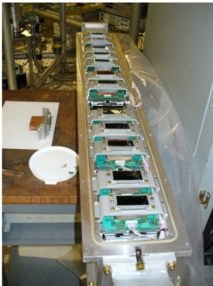
UCN detector with analysis of polarization (13 neutron channels, 117 Si detectors with electronics)
