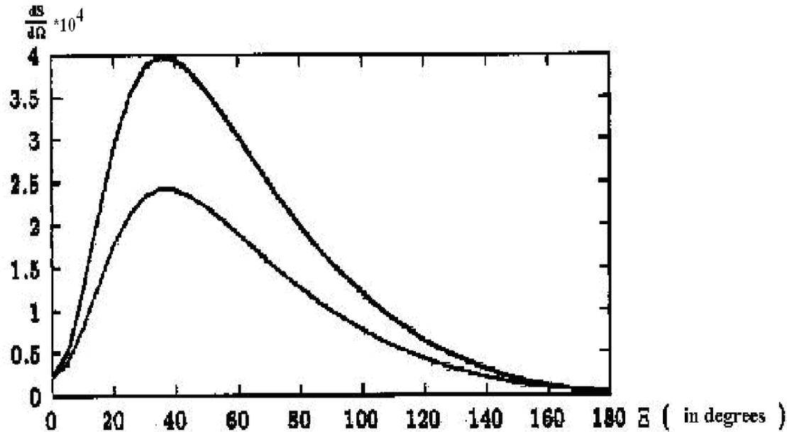
Dependence of the radiative decay spectrum  $S$  on the angle  $\Xi$  between the photon and the electron momenta (upper curve for a threshold gamma energy of 25 keV, lower curve for a threshold gamma energy of 50 keV)
