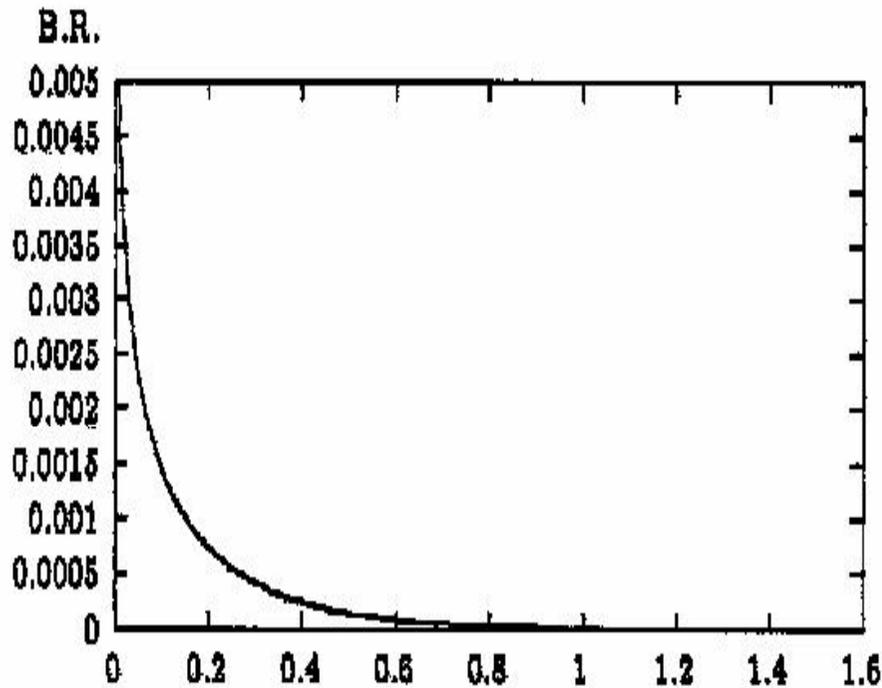
The expected Standard Model branching ratio for radiative neutron beta decay (summed over all gamma energies larger than the threshold gamma energy  $\omega$ ) as a function of  $\omega/m_e$ .
