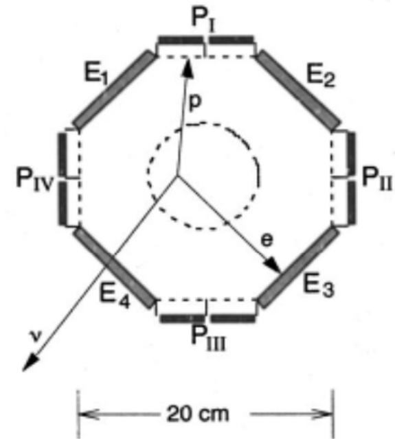
Schematic lay-out of experimental setup
