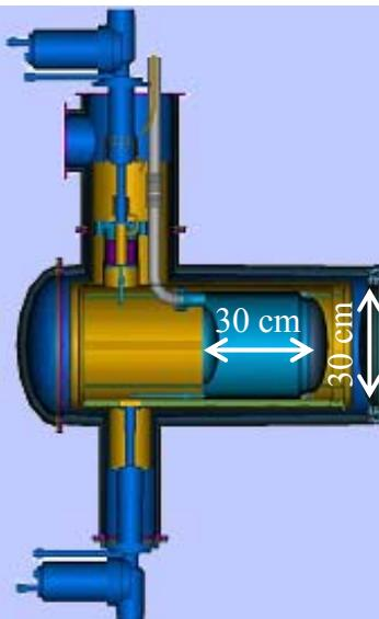
16L vessel of liquid parahydrogen
